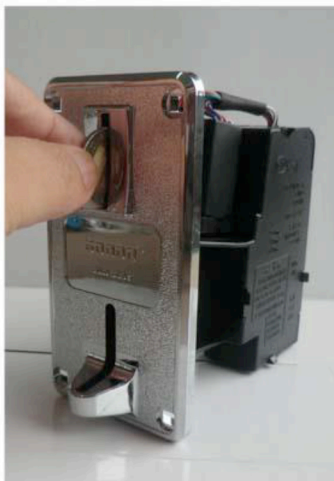
3rd step: drop coin 30 times until LED off
