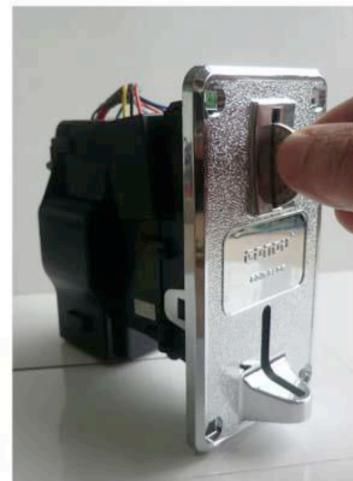
3rd step: drop coin 30 times until LED off
